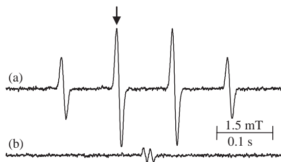
Figure 1. Stopped-flow ESR spectra recorded by field-sweep mode. (a) ESR spectrum recorded by mixing the sonicated DMPO solution (0.2 mL) and buffer solution (0.2 mL), (b) ESR spectrum recorded at 5 s after mixing solutions of DMPO/OH (3.1 \mu\text{M} , 0.2 mL) and ascorbate (100 \mu\text{M} , 0.2 mL). The concentration of DMPO/OH and ascorbate correspond to the initial concentration just after mixing. The downward arrow indicates the static magnetic field for the stopped-flow ESR measurements by time-sweep mode.
